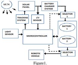
The framework for system is shown in figure1.[3] System contains The robotic vehicle developed to be guided and has a set of four wheels coupled to a plane chassis that can rotate independently and the individual control of each
